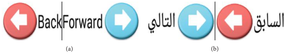
FIGURE 3: Snapshot of a direction-sensitive arrow that changes meaning when mirrored. (a) UI in English. (b) RTL UI.
