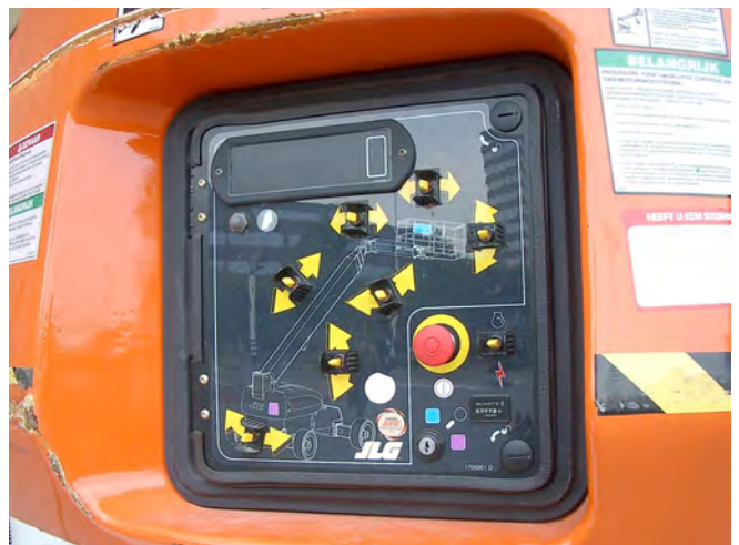
Figure 4: A graphical variant of natural mapping: the controls are placed in a perspective linedrawing of the crane itself.
