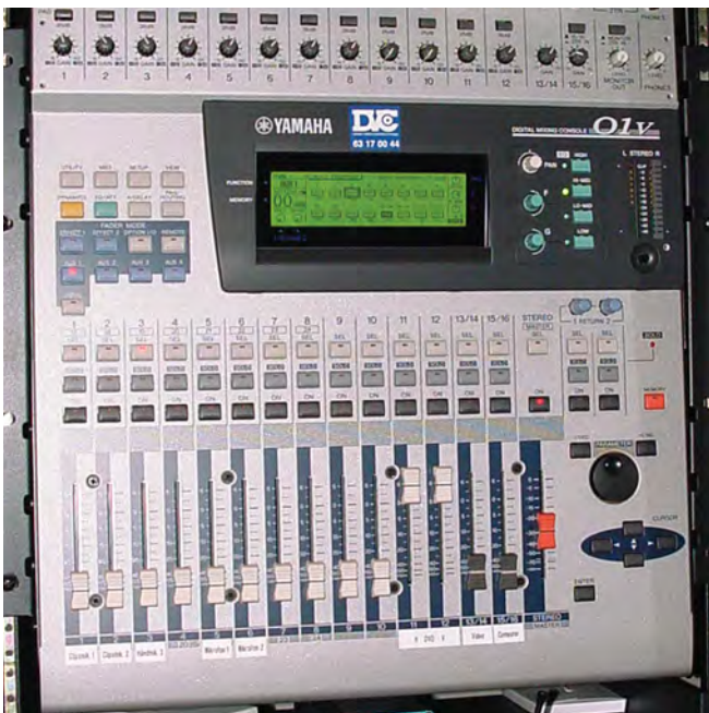
Figure 2: In most electronic products the controls clearly communicate the required actions (pushing, sliding, rotating etc.) but this does not necessarily mean that they communicate their function.
