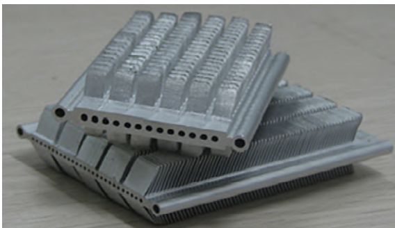
Fig. 1. Integrated fin and micro-channel heat exchanger core section.
