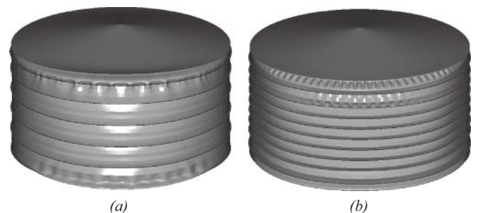
Fig. 26. The failure modes of Tank D for horizontal rings every (a) 4 m and (b) 2 m.
