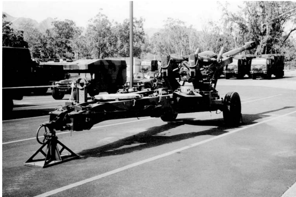
Fig. 8 M198 howitzer in “ready” position. Source: Ref 5
