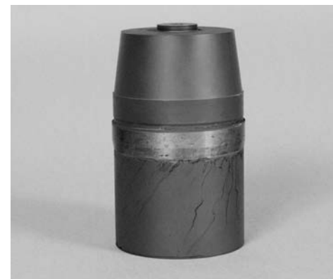
Fig. 4 Galvanic corrosion at the interface of the copper rotating band and the steel base metal in a 105 mm cartridge. Source: Ref 3
