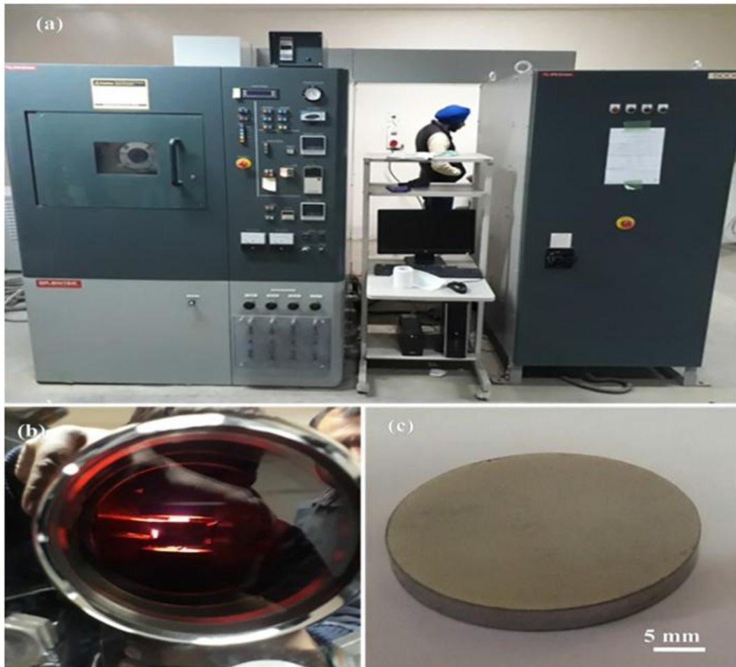
Fig. 2. (a) Spark Plasma Sintering machine (S-5000), (b) red hot sample under vacuum during the process, (a) and as-consolidated sample. (For interpretation of the references to colour in this figure legend, the reader is referred to the web version of this article.)
