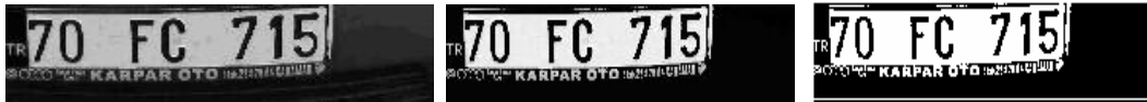
Fig. 3. (a) original plate region image; (b) contrast extended image; (c) median filtered image
