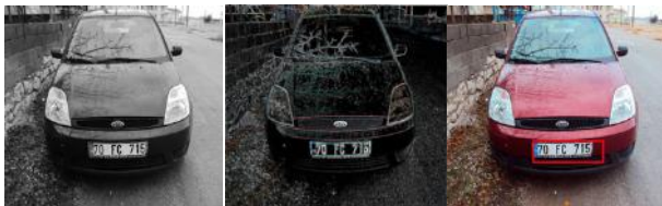
Fig. 2. (a) original car image; (b) edge detected; (c) localized plate region
