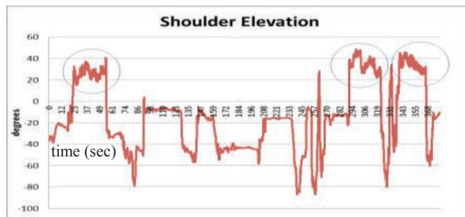
Fig. 4. Graph of upper arm elevation during 6 minutes of sanding drop-down panels overhead. The circled areas are continuous period of overhead sanding.
